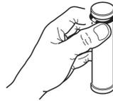
Pinch the part and the seal between the thumb and index finger; push it back towards the opposite side to deform it.
