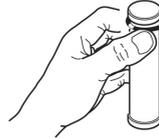
Accentuate the deformation to take hold of the section of the seal which overlaps, then remove the seal from its bearing.
