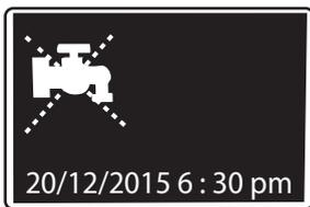
This alarm appears if the REC recording function is active when the pump water meter and the flexible blade switch cycle counter sends no pulse for 30 minutes (value pre-defined in onboard software). E.g. DOSATRON bypass valve remained accidentally closed or break in water supply (network problem, filter blocked, etc.)
