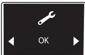
● Pressing the validation button again removes the alarm and reinitialises the maintenance meter
