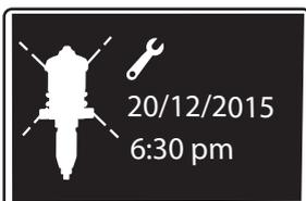
The water circulates, the water meter detects the flowrate but the Dosatron pump motor is shut down (no signal detected by the flexible blade switch sensor located on the doser lid).
